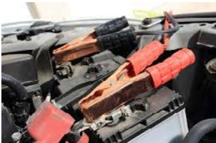
Explosive hydrogen... acidic liquids and vapors... electrical burns... strains, sprains, hernias, and compressed discs. All of these hazards arise when servicing, charging, or jumping the common lead-acid battery found in cars and trucks. The hazards can be minimized by following a few common sense safety rules.
