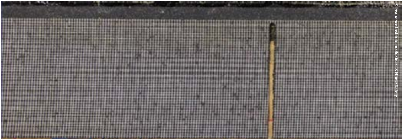
Figure 1: Example of mesh on the back of an IR 3-tab shingle.
